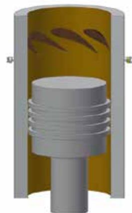
Cylinder oil injection before piston passes = thin and uniform oil film
