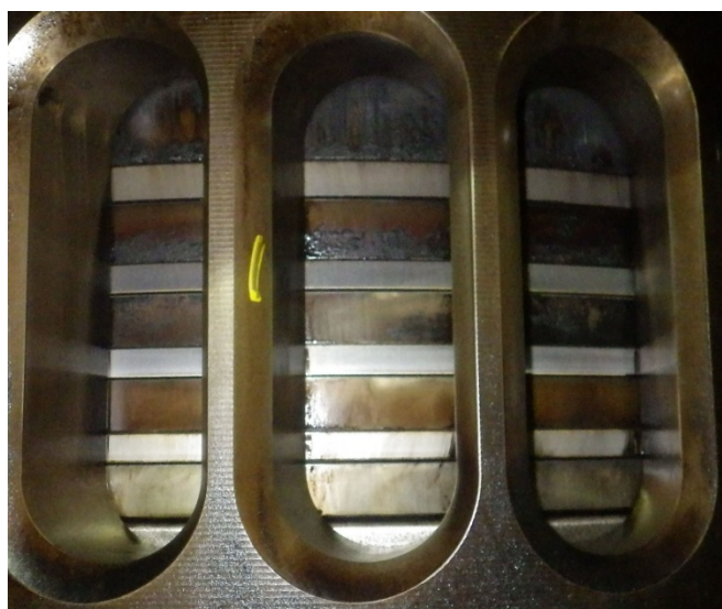
Figure 13: Piston ring condition on unit number 1 after 10319 running hours.
